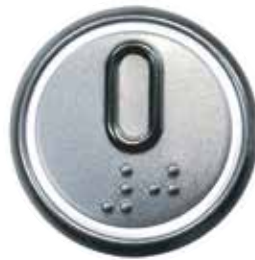
RDV Diameter 33.8 mm EN81.70 Braille 24V, NO Lighting Colour: White
