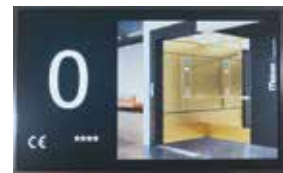
TFT 5 Colour Screen (Res: W 800px H 480px, Colour Depth 24-bit) Floor Number & Direction Arrows Time-Date-Temperature Floor Logo pictures and specific pictures for modes of operation (Overload/FireAlarm/Service) Eco mode (for lower power consumption) 2 Languages (English-Greek)
