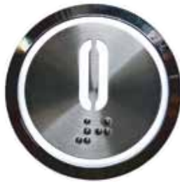
RDB Diameter 36mm EN81.70 Braille 24V, NO Lighting Colour: White
